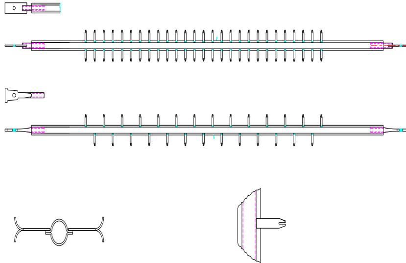
Figure 2 –Aggressive and Standard ELEX Electrode
